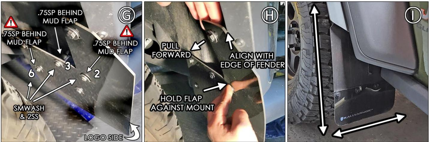
**REAR FLAP** Tighten fasteners just enough to allow for adjustment later. **Bracket/Hardware 1 x FLAP → 1 x BMF84-LR2/RR2**
